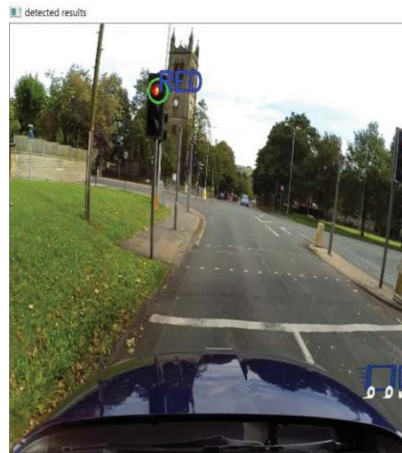
FIGURE 1: The Red Color Traffic Signal is Detected.
